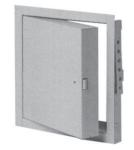
For vertical wall applications. Features 16-ga. steel frame, 18-ga. steel door, 1-7/8" mineral wool insulation, concealed pivot-type hinge, automatic closer and inside release. 140° opening angle. Self-latching. Gray enamel finish. UL and Warnock Hersey listed.
