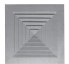
Designed to visually complement modular ceilings. Provides consistent flow pattern throughout CFM range; ideal for use in variable air volume (VAV) systems. 22-ga. metal border with removable core. White finish. **Fixed Discharge.** Horizontal pattern only. **Adjustable Discharge.** Features movable vanes for changing pattern
