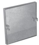
For use with steel ductwork. Manual locks provide secure closure. Features 22-ga. steel frame; cammed, removable double-skin door; foam gasket seal and 1" thick fiberglass insulation.
