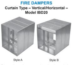
For use in static systems that shut down during fire. Can be installed vertically in wall or horizontally in concrete floor. Features 12" 20-ga. galvanized steel sleeve, 24-ga. galvanized steel blades, picture frame mounting angles (2 sides) and 165°F fusible link. UL and CUL classified. FM approved.
