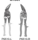
Compound leverage. Capacity 18-ga. cold rolled sheet metal; 22-ga. stainless steel. Serrated, alloy steel blades with grade-8 center pivot bolt and double-overwind spring. Molded plastic grips. Overall length 9-1/4". Cut length 1-1/4". Meets ANSI specifications.
