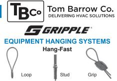
Provides lighter, easier and faster alternative to threaded rod for hanging mechanical, electrical and HVAC equipment. Ready to use; requires no additional preparation time. Includes cable with loop or stud end fixing; grip secures free end of cable and allows height adjustment of hanging object. **Loop.** For wrap-around anchoring on bar joists or other roof structures. **Stud.** For anchoring into concrete or metal. metal. Includes 1/4" drop-in expansion anchor.
