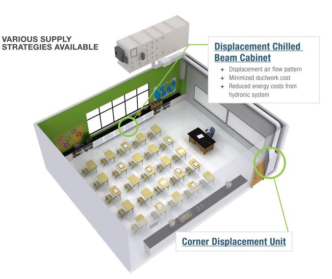
Displacement Ventilation operates on the same principles as UFAD supplying air directly into the occupied zone and creating stratification. Typically diffusers are ducted from the ceiling to a low level supply diffuser. In some cases ceiling diffusers can be used to free up wall or floor space.
